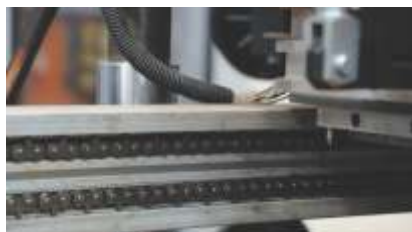
Servo controlled frictionless chain transport
